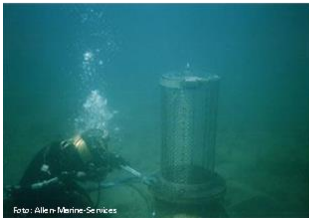
Figure 24: A diffuser that can prevent a diver from getting trapped
