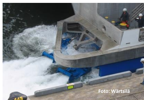
Figure 11: Propulsion through Waterjet's systems
